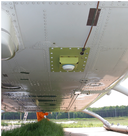
Fig. 8. Pseudolite antenna underneath the MH2000A.
