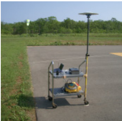
Fig. 12. The rover which consists of the GPS/PL receiver, antenna, PC, and battery.
