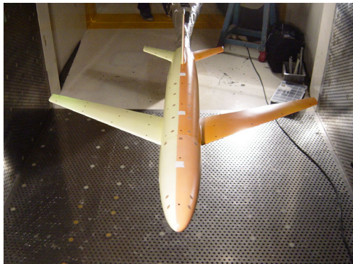
Fig.7. PSP/TSP Painted ONERA M5 Model Port Side(pink): PSP Starboard Side(yellow): TSP
