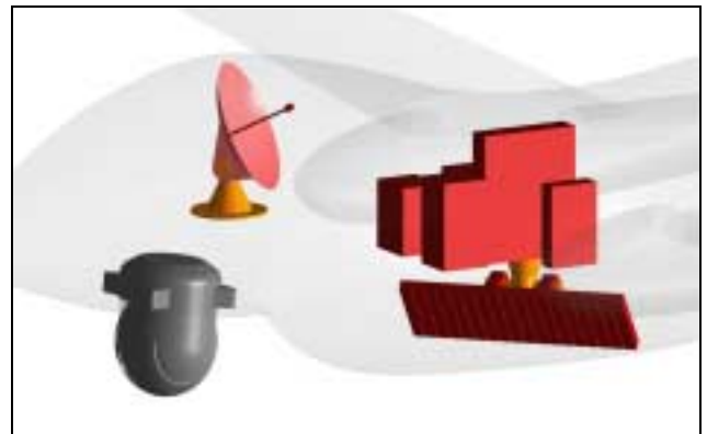
Fig. 24 - FLIR head, SAR and SATCOM antennas arrangement in the UAV3 General Preferences
