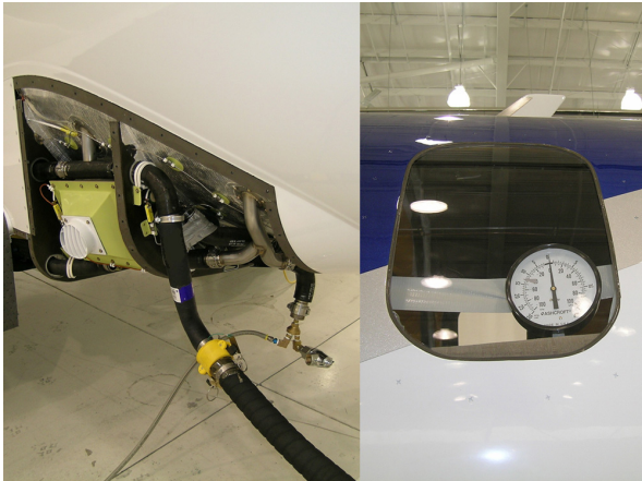
Fig.16. Ground pressurization tests.
