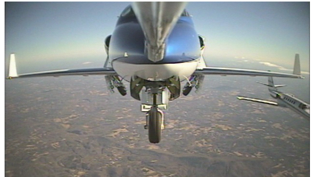
Fig.7. Landing-Gear operation test.
