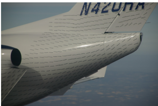
Fig.17. Flow visualization using tufts
