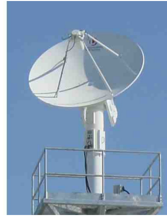
Fig. 3. Automatic tracking antenna.
