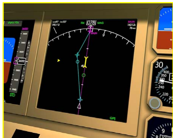
Fig. 2. Illustration of conflict alerting and strategic resolution advisory from an integrated AOP system.
