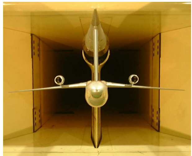
Fig. 21. The Model with Nacelles for KTWT Wake Survey.
