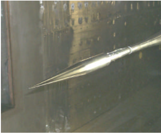
Fig. 4. Ten-Degree Cone Probe Installed in the Solid Test Section
