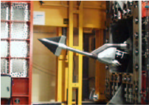
Fig. 1. Generic delta wing and model sting with roll drive unit in the wind tunnel setup
