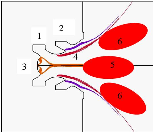
Fig. 15. Basic principles for multipoint injection systems. 1: primary swirler, 2 secondary swirler, 3 fuel injection for low rating, 4 fuel injection for high rating. 5: combustion zone for low rating, 6: combustion zone for high rating
