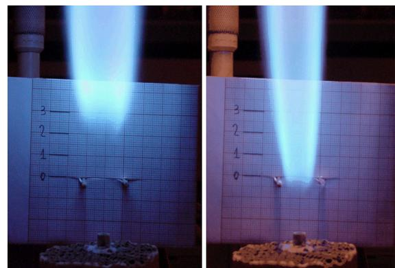
Fig. 17. Illustration of the plasma effect on a flame stabilization problem. Left: no plasma is applied and the flame is near the lean blow out limit. Right: only plasma is applied and the flame become perfectly stable. (Thanks to CNRS / CORIA for the picture)
