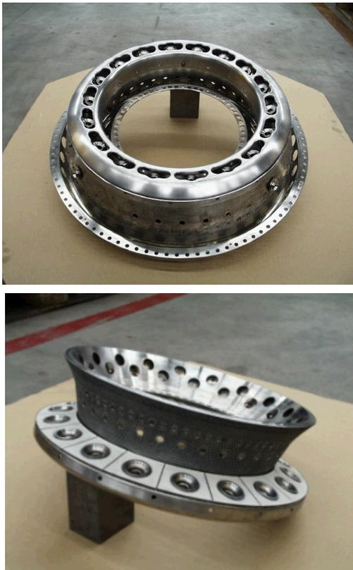
Fig. 11 DEM21 combustor and the inner liner
