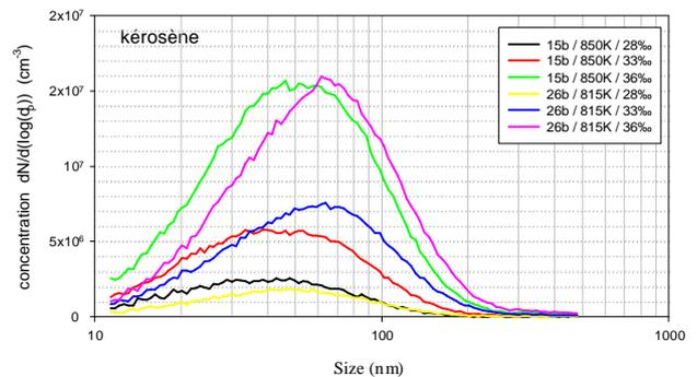
Fig. 3. Particulates size distribution on Snecma Moteurs prototype combustor
