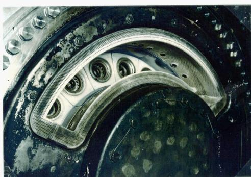
Fig. 16. The SNECMA Moteurs variable geometry injection system multi-sector combustor
