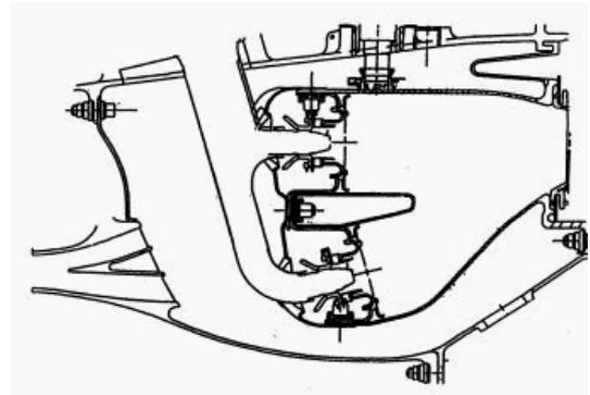
Fig. 12. SNECMA Moteurs DAC combustor demonstrator (civil project PAT - 1997)
