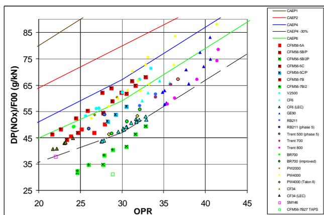
Fig. 7. In production certified engines
