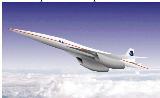
Fig. 2 Image of NEXST2: jet-powered supersonic experimental airplane.
