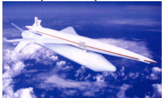
Fig. 1 Image of NEXST1: non-powered supersonic experimental airplane.
