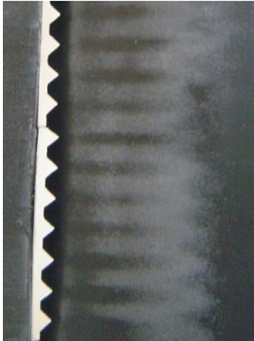
Fig.14. Visualization effect of saw-tooth on upper surface flap at Re = 400000 . \alpha = 10 -deg and flap at 12-deg.
