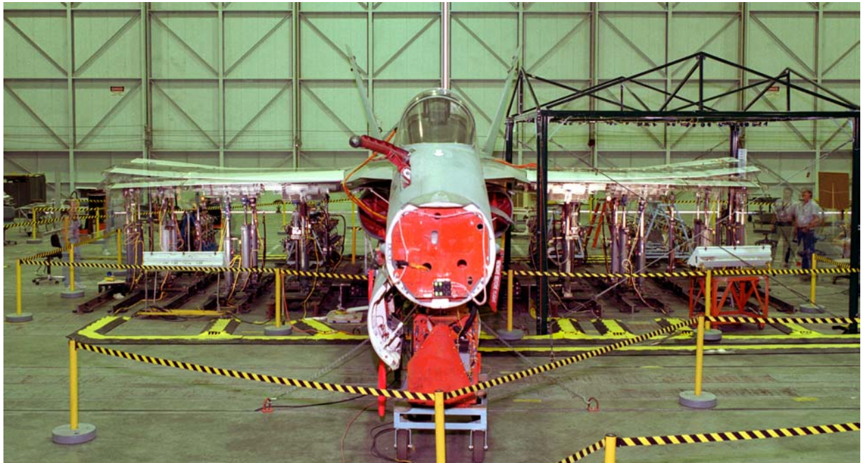
Fig. 5. Composite photograph of AAW aircraft undergoing distributed loading at zero load and at maximum up load.
