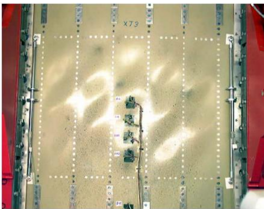
Fig. 17. Buckling Pattern in the Physical Test (Photo)
