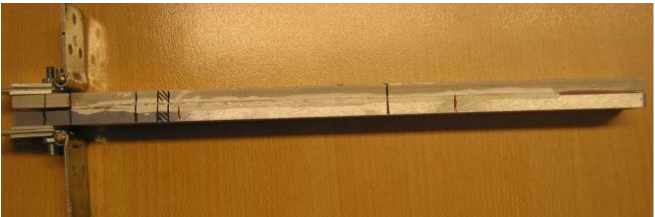
Fig. 3. Test specimen: hinges attached (left), white fluid painted on edge for crack growth monitoring
