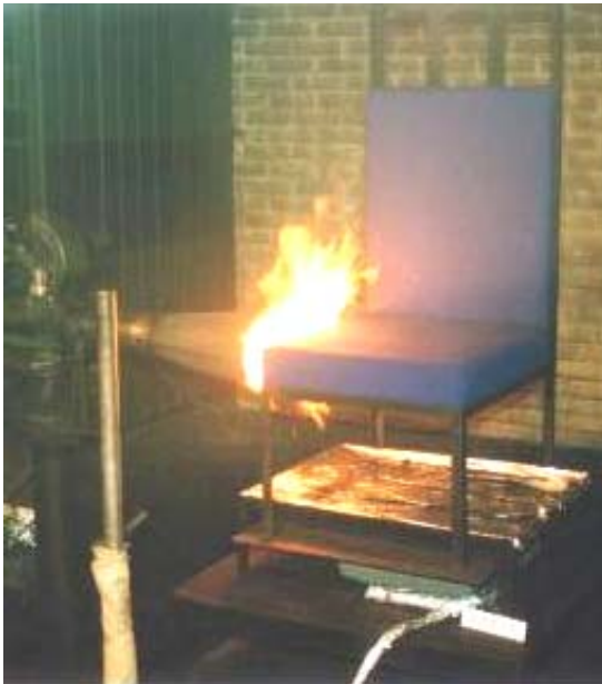
Fig. 3 Cushion Flammability Test
