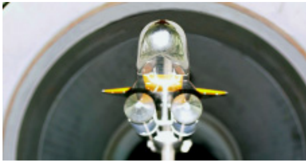
Fig.13 TSTO Model in NAL M10 HWT
