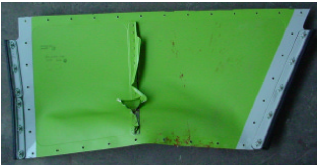
(b) Inside of Pylon Cover and Stiffener
