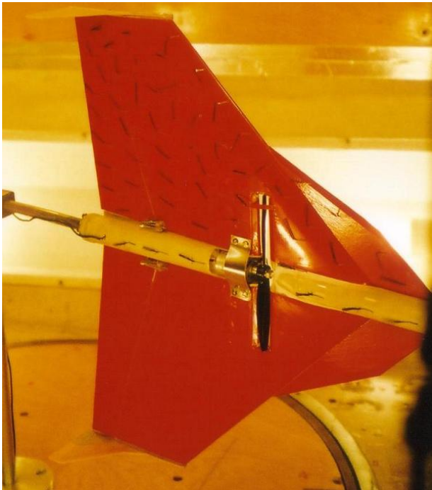
Fig.16 Propeller effect for angle of attack of 20°.
