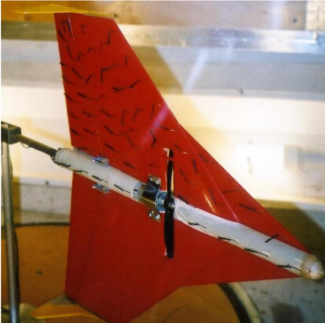
Fig.18 Propeller effect for angle of attack of 30^\circ .
