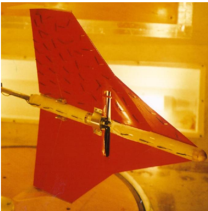
Fig.17 Propeller effect for angle of attack of 25°.
