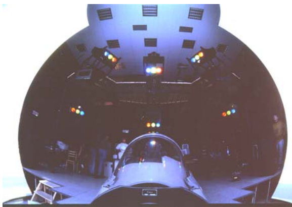
Fig. 6. The 6-channel projection system and a spherical screen (backward view)
