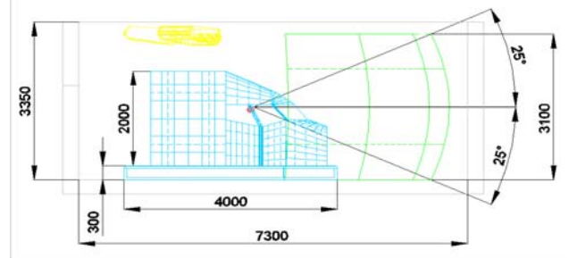
Fig. 2. General simulator cockpit layout
