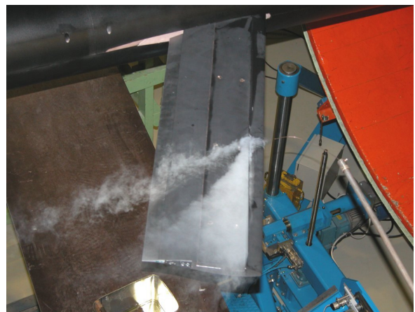
Fig.11b: Effect of no rear fence – outboard end of double-tooth front fence
