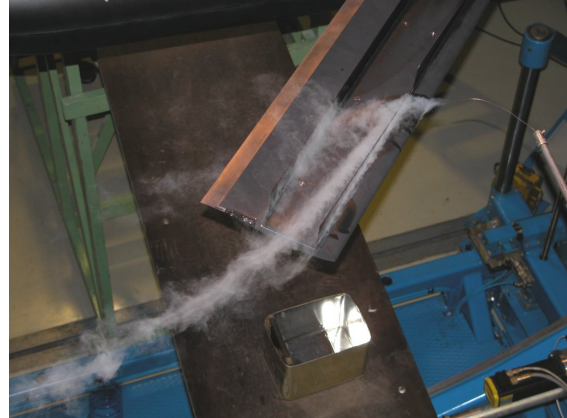
Fig.8b: Vortex generated by outer tooth of double-tooth front fence
