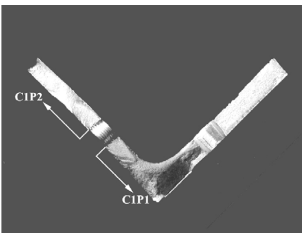
Fig. 10. Fracture surfaces of cracks C1P1 and C1P2 initiated on the rivet hole in lower flange plate.
