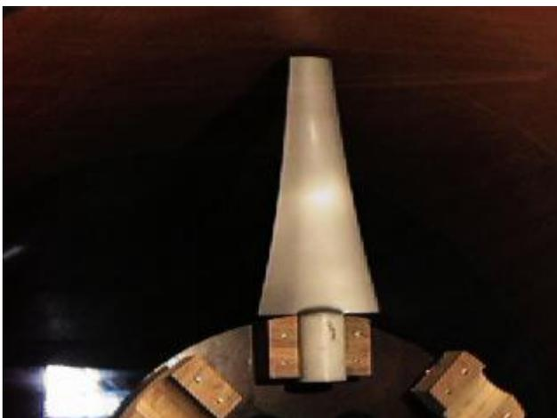
Figure 9 Blade/boss assembling.
