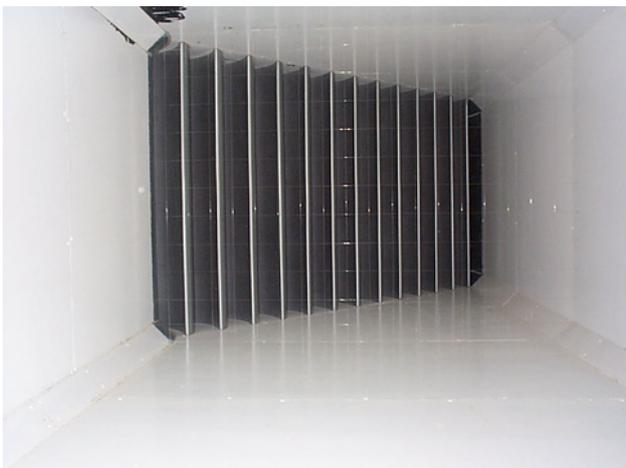
Figure 8 First corner vane section.
