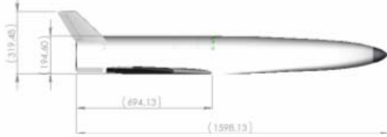
Fig. 6: side view of the Mini-FTB
