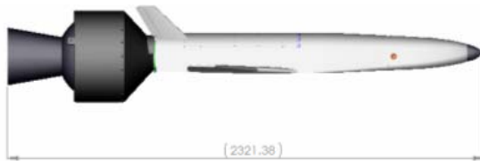
Fig. 7: side view of the Mini-FTB and its propulsion system
