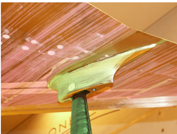
Fig. 8 Oil flow visualisation near the pylon at design lift: \alpha_{exp} = 10.5^\circ
