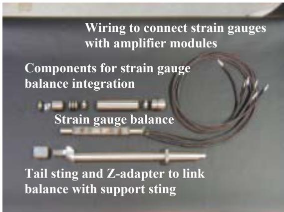
**Fig. 6** Components for strain gauge balance integration and connection with tail sting adapter.
