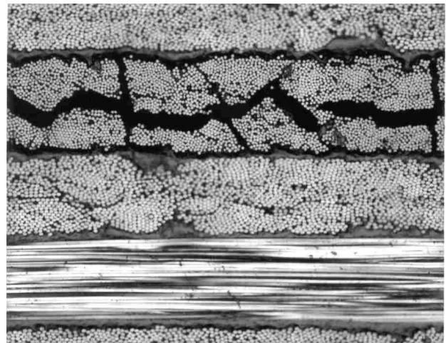
Fig.3. Damage observed on 3 plies of a [+45/0/-45/90]4s QI carbon fiber/ BMI resin composite after aging at 180°C/6000 h. Only 0° ply is microcracked.
