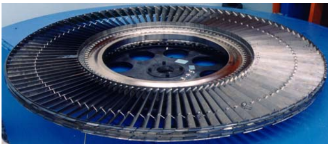
Fig. 3: LP turbine stage of the GE CF6-80C2 jet engine with turbine blades manufactured from a cast Ti-47Al-2Cr-2Nb alloy (courtesy GE Aircraft Engines, USA)
