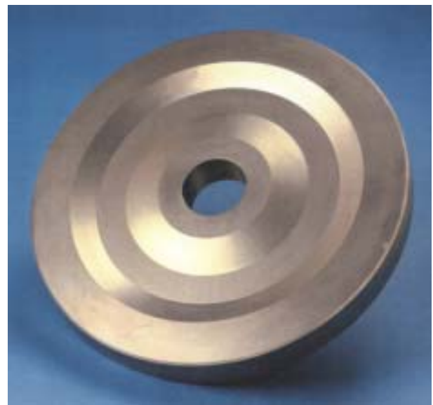
Fig. 1: Machined compressor disk „Stage 3 blisk“ made from TIMETAL 834; 40kg weight; 500 mm diameter (courtesy Otto Fuchs, Meinerzhagen, Germany)
