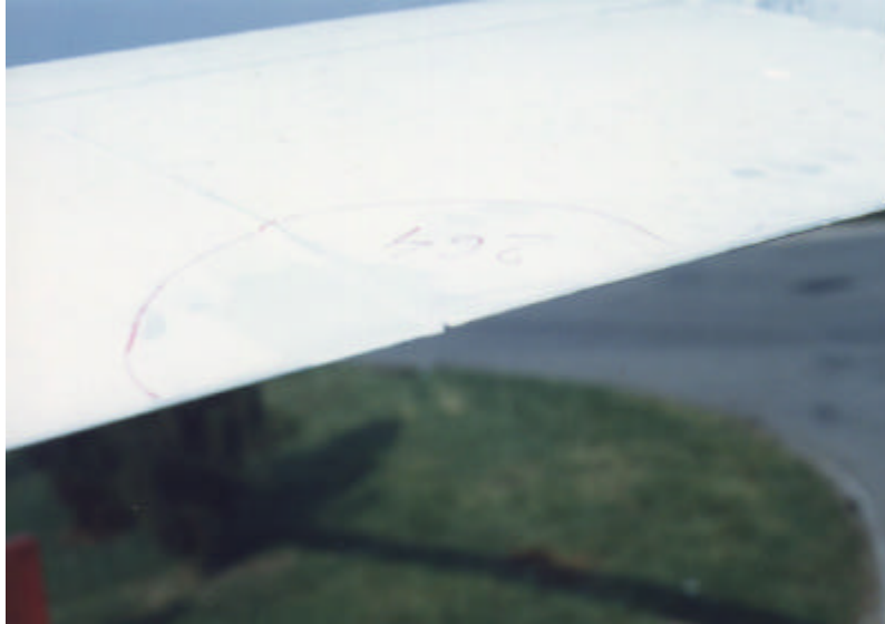
Figure 3. Ballistic damage of the main rotor blade.
