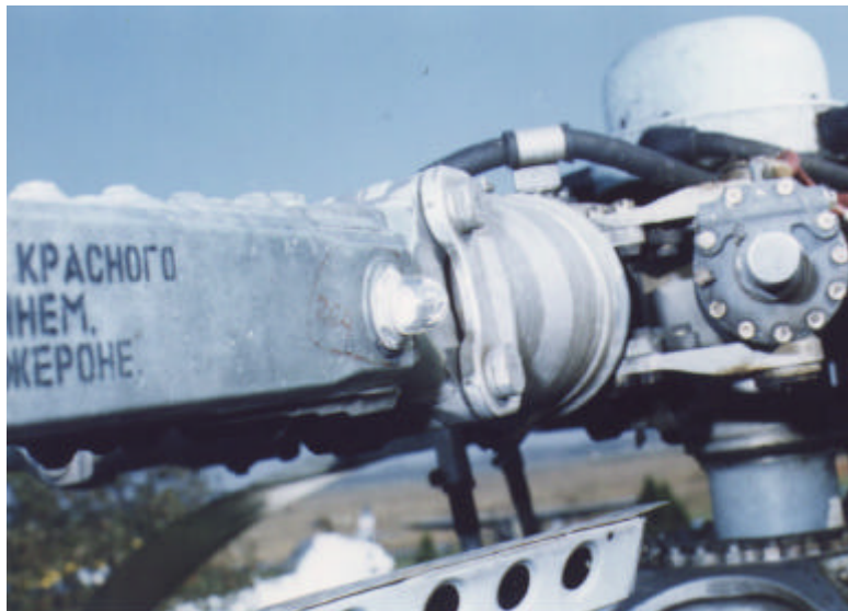
Figure 4. Ballistic damages of transmission and main rotor head.
