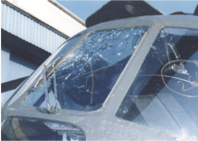
Figure 2. Ballistic damages of helicopter's windshield.
