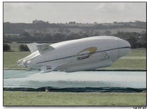
Fig. 2. SkyKitten 1, 1/7 th scale model of SkyCat™ 20.
