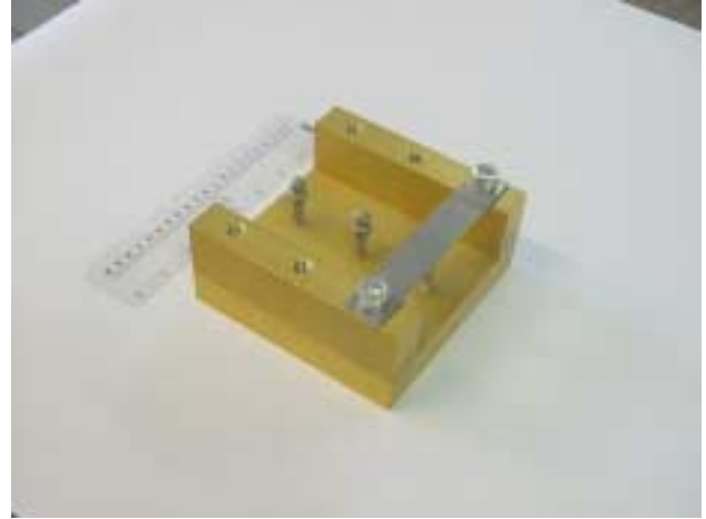
Figure 3: EB Vareststraint Test Fixture and (P) Loaded Specimen
