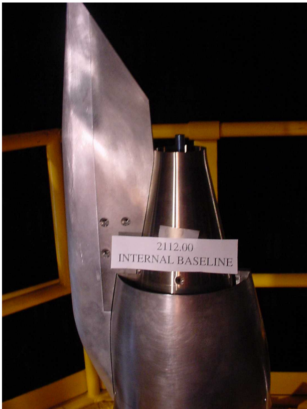
Figure 5 Photograph of CFM56-5B conventional exhaust system scale model.
