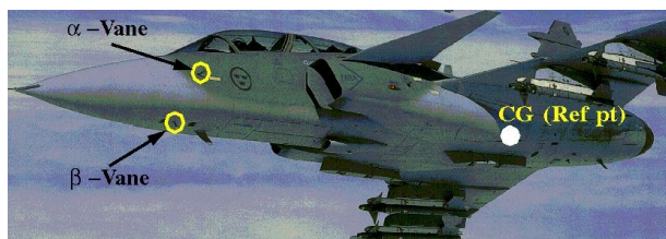
Figure 4. SAAB 39 Gripen with reference positions of weather vanes and center of gravity (CG) indicated
