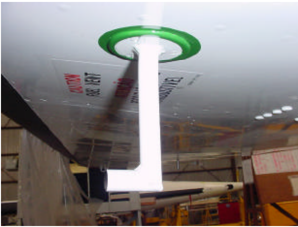
Fig. 1. Vent tube of the wing fuel tank.
