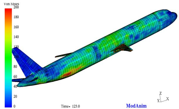
Figure 15 : Von Mises Strength (ALE)
