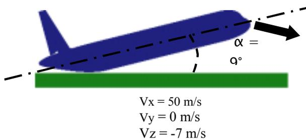
Figure 11 : Ditching configuration
