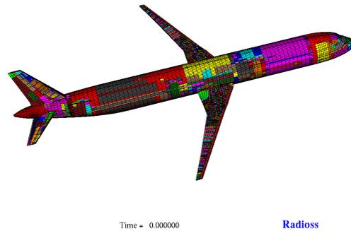
Figure 10 : Airbus A321 mesh model
