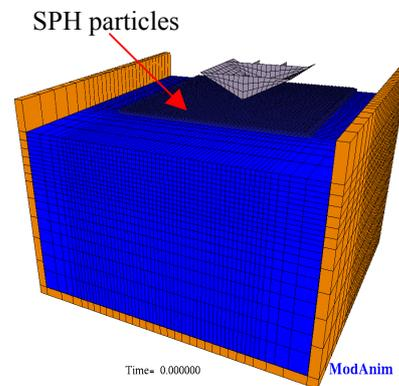
Figure 7 : Hydrodynamic tunnel modeling (SPH)
