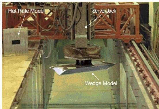
Figure 1 : Hydrodynamic tunnel and servo jack
