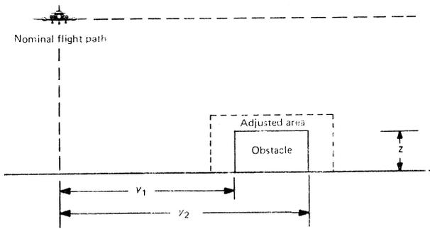
**Fig. 8: Adjustment of object dimensions based on aircraft dimensions (Ref.: [5])**
