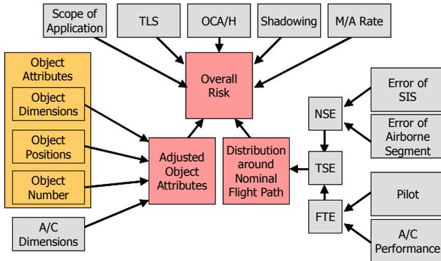
Fig. 10: System elements of a GBAS CRM (own figure)
