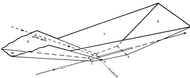
**Fig. 2: Protected airspace for precision segment of ILS approaches – Obstacle Assessment Surfaces according to ICAO PANS-OPS (Ref.: [4])**
