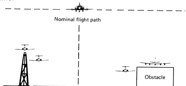
Fig. 7: Dimensions of aircrafts and objects for risk calculation (Ref.: [5])
