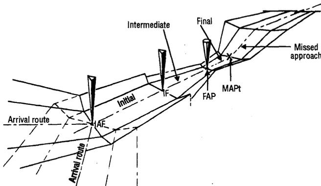
**Fig. 1: Segments of an instrument approach according to ICAO PANS-OPS (Ref.: [4])**
