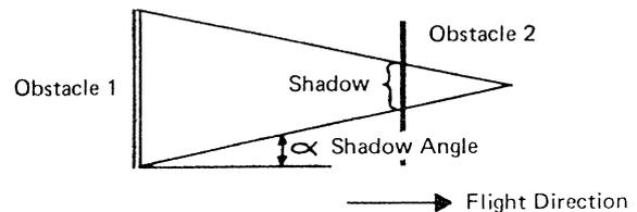
**Fig. 9: Principle of shadowing (Ref.: [5])**
