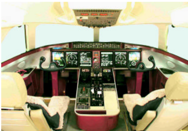
Fig. 16 Most modern Cockpit Concept with highly integrated utility management system for reduced workload, increased flexibility and optimized maintenance
