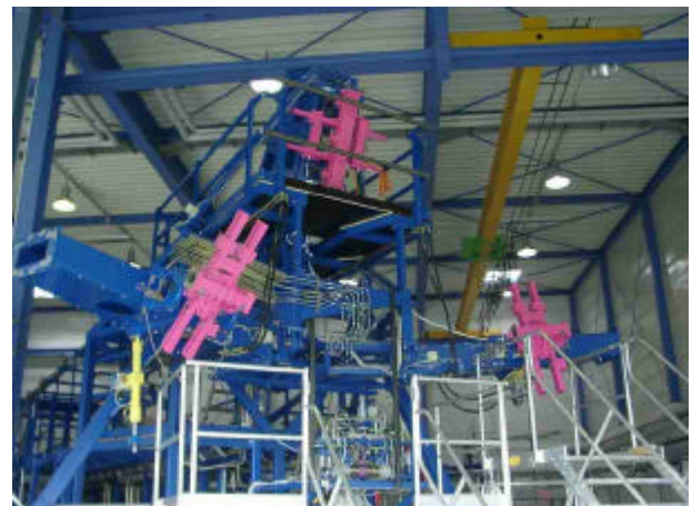
Fig. 17 Horizontal and vertical tail on the Iron bird with actuators, simulated surfaces and artificial load system
