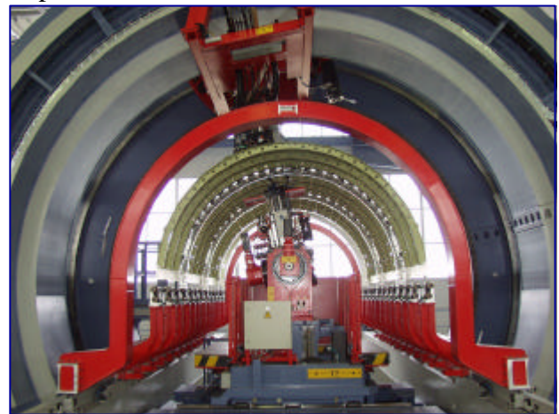
Fig. 20 728 Family Fuselage Automated Riveter
