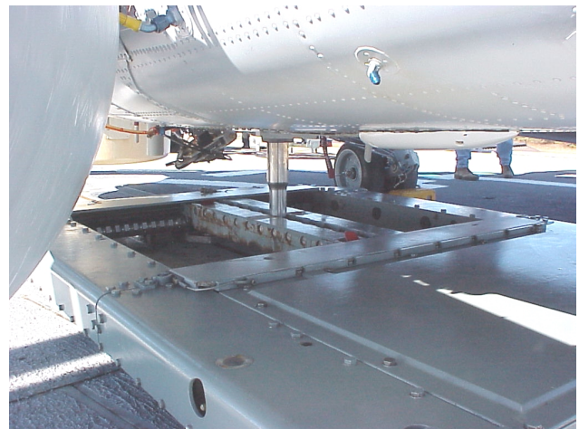
Figure 13. SH-2G(A) Aircraft in the RSD During Operational Testing.
