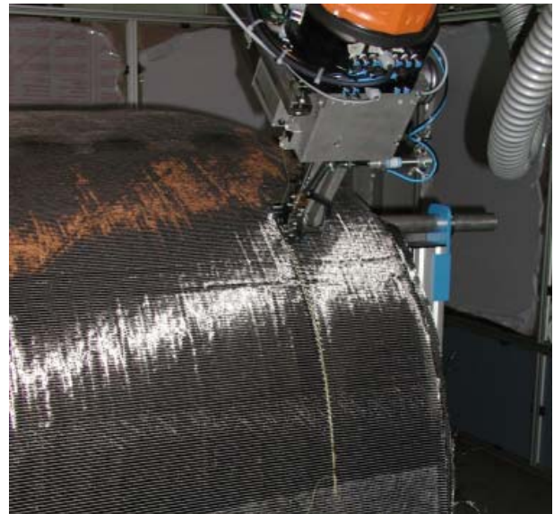
Figure 11. First blind stitch seam after skin lay-up
