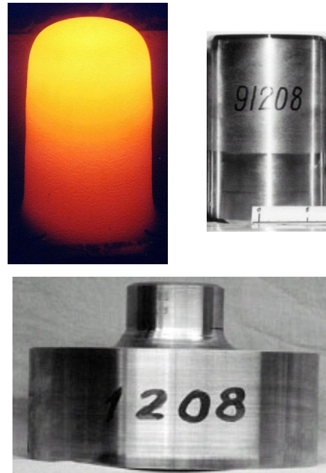
Fig. 4. As-spray formed billet (upper left), machined pre-forged cylinder (upper right) and forged disk part (lower) of a high performance superalloy.
