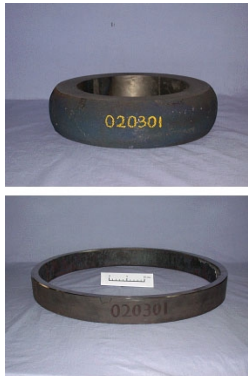
Fig. 5. Spray formed ring perform (upper) and rolled ring (lower).
