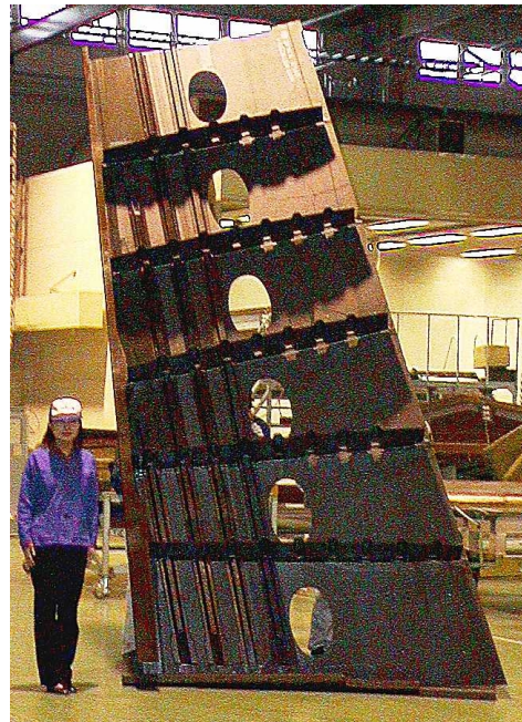
Co-bonding of Skin, Stringers and Rear Spar
