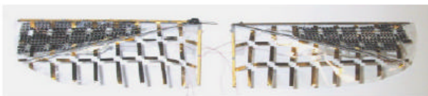
Figure 9: Wing with integrated MEMS checkvalve electrostatic actuators
