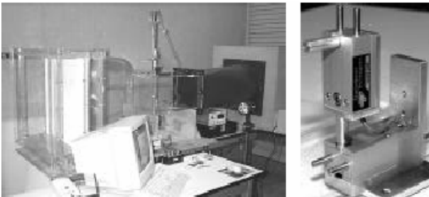
Figure 1: Wind tunnel and test stand load cells
