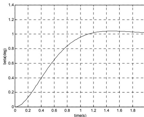
Figure 5: Ideal model response of the sideslip at step input.
