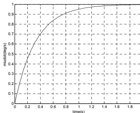
Figure 6: Ideal model response of the stability axis roll rate at step input.
