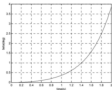
Figure 3: Sideslip response to step input (without controller)
