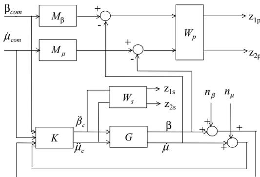
Figure 1: Model matching control configuration
