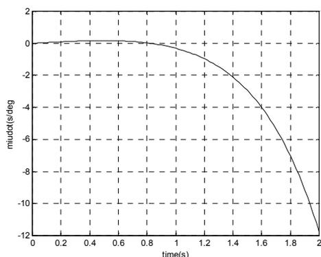
Figure 4: Stability axis roll rate to step input (without controller).
