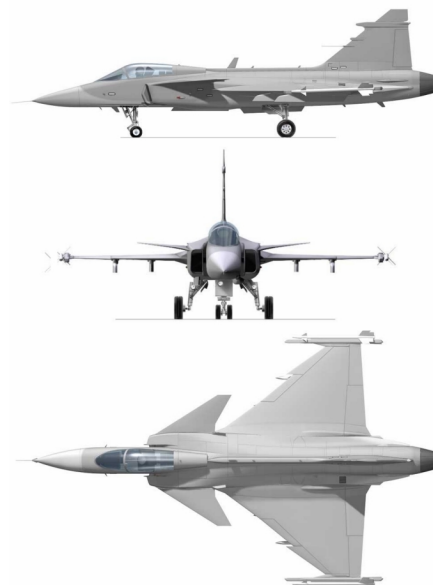
Figure 1. Three-view layout of the Gripen 39A single seater.
