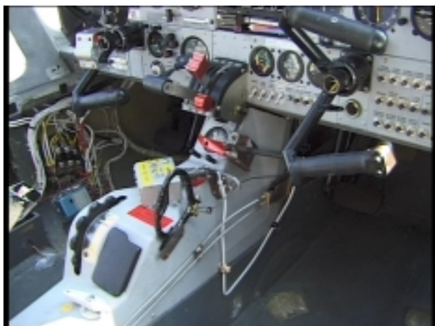
Fig.13 Cockpit of the Manager Aircraft. In emergency the black ring handle can deploy the auxiliary parachute, the red handle (right and above of the black ring handle) after recovery allows throwing away the main parachute
