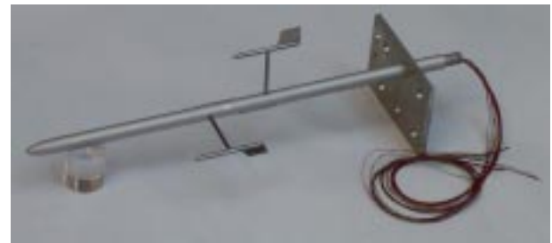
Fig. 12. Probe for the measure of the angles of attack and of sideslip.
