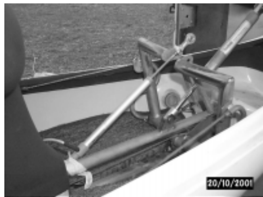
Fig. 11. Potenziometer for the measure of rudder angular deflection, as installed on a DG400 sailplane.
