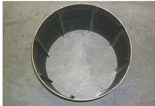
Fig. 2. Top view of a stiffened cylinder.
