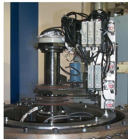
Fig. 4. Equipment for the measurement of the post-buckling mode.
