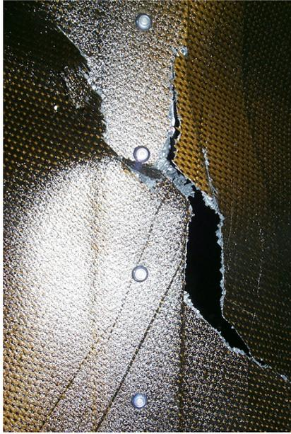
Fig. 13. Photo of the failure of a stiffener.
