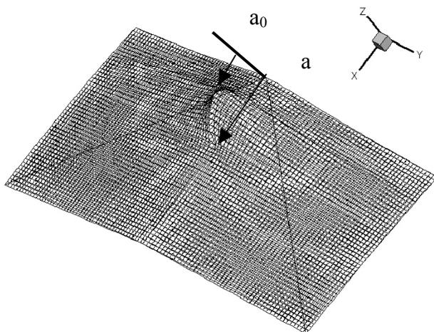
Fig. 6. The in-plane displacement discontinuity at the interface, which is believed to be the cause of delamination.
