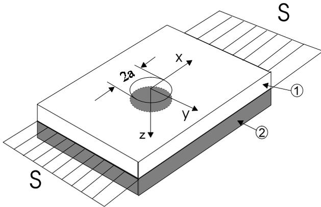
Fig. 2. A three layer FML containing a circular hole, remotely subjected to a uniform stress  $S$ .
