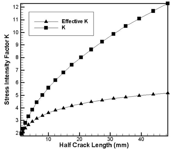
Fig. 5. Comparison of stress intensity factors in bare metal and FML.
