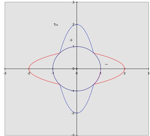
Fig. 3. Distribution of the inter laminar stress  $\tau_{rz}$  around the hole of  $a = 1$ . The abscissa is parallel to the x-axis and the ordinate is parallel to the y-axis. The maximum interlaminar shear stress is normalized to be unity.
