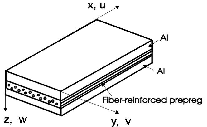
Fig. 1 Schematic of a three-layer FML.
