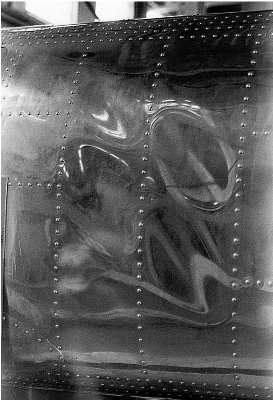
Fig. 2. Diagonal tension in a Canadair CT-114 Tutor
