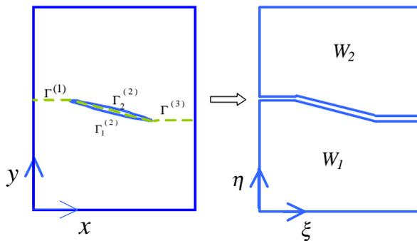
Fig. 2 Solution scheme for a cracked plate
