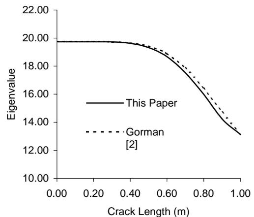
Fig. 6 Eigenvalue vs. for a plate having a central crack emanating from an edge
