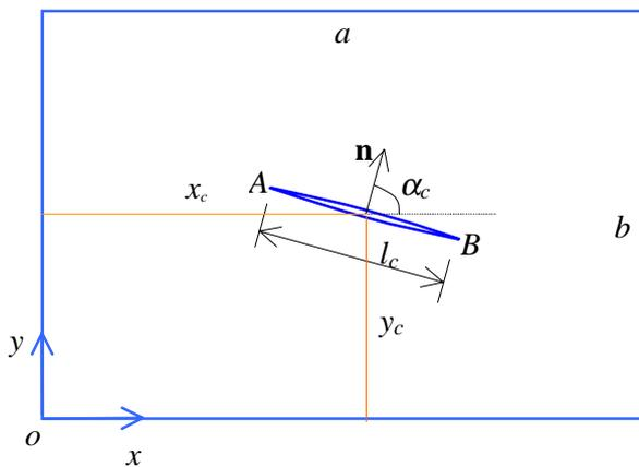
Fig. 1 A rectangular plate having a linear crack
