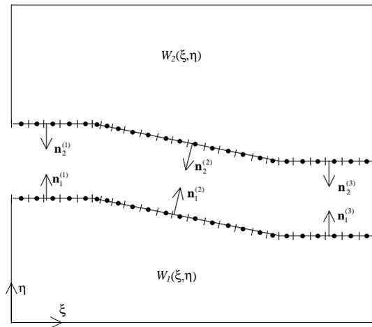
Fig. 3 An illustration of line boundary element mesh along the interface
