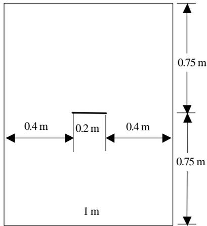
Fig. 4 A simply supported plate having an internal central crack ( $h = 0.05$  m,  $E = 69$  GPa,  $\nu = 0.3$ )
