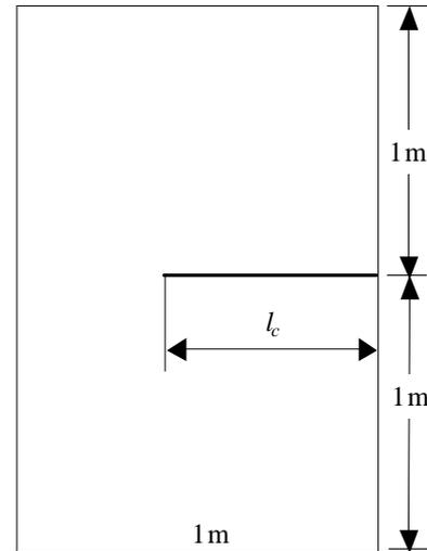
Fig. 5 A simply supported plate having a central crack emanating from an edge ( $h = 0.05$  m,  $E = 69$  GPa,  $\nu = 0.3$ )
