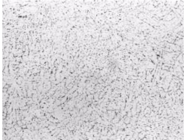
Fig. 6 Transition from Columnar to Equiaxed Dendrites near Weld Centreline (6013 with 5556 Filler Wire)
